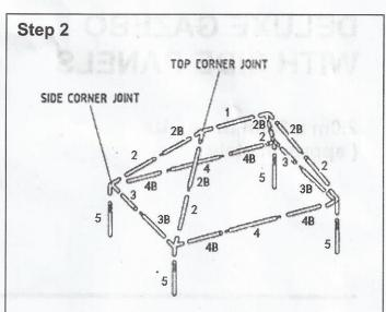
Assemble the frame top and half the legs using - Tubes, 1, 2B, 2, 5 & the Top Corner Joint.
