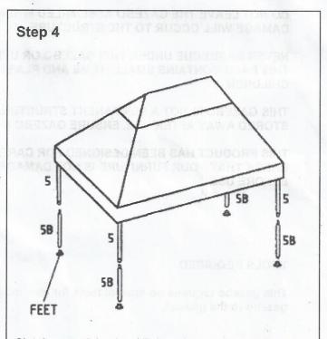
Slot the remaining leg (  $\mbox{Tube 5}$  ) into position. Push the plastic feet into place.
